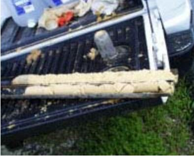
Split-spoon sample during drilling of monitoring wells typifies the uniformity of the sandy deposits on the Ridge. - [click to enlarge](#)
