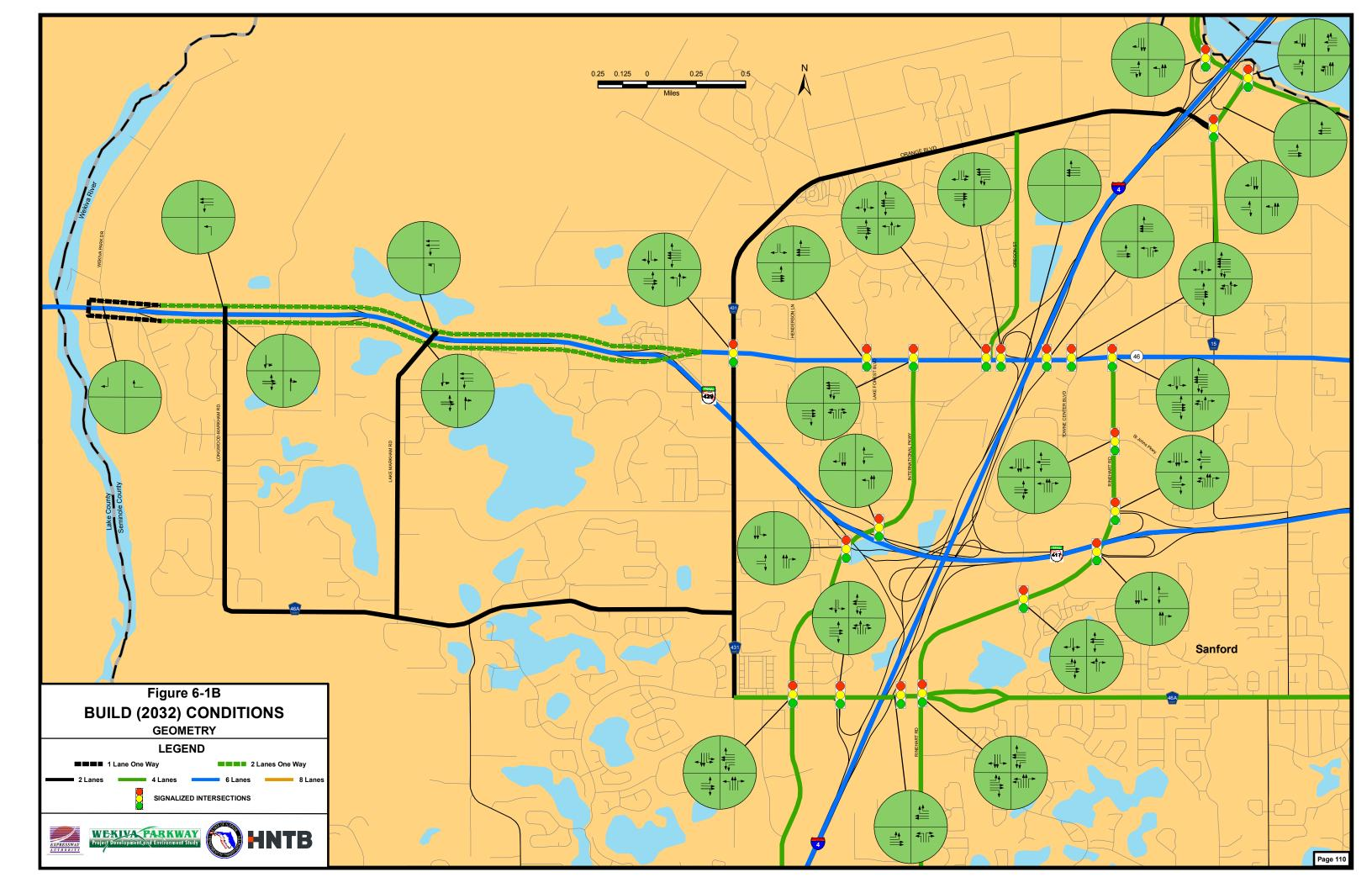
While the recommended configuration of these three local access interchanges was for a full western interchange and a split diamond interchange between the central and eastern interchanges, the preferred alternative includes three full interchanges due to the environmental concerns associated with keeping a remnant of existing SR 46 open to connect the central and eastern interchanges.
