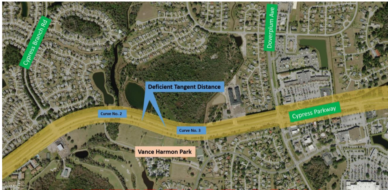
Figure 6.5.1: Deficient Tangent Distance Between Curve Nos. 2 and 3
