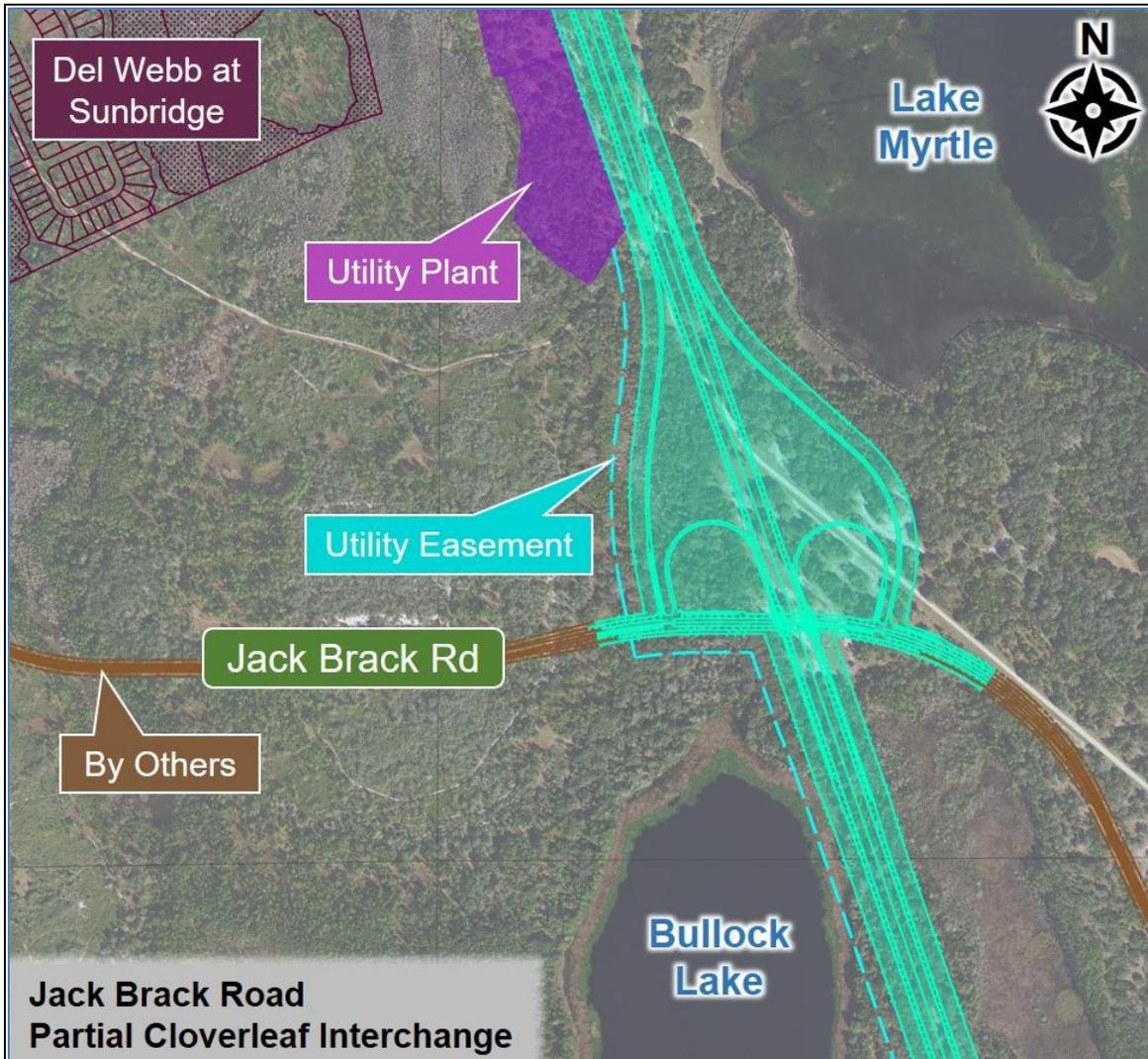
The Diamond Interchange as shown on **Figure 1.1.4** has exit ramps in the southeast and northwest quadrants of the interchange that will allow for traffic exiting the expressway to continue east or west along Jack Brack Road. There are also entrance ramps in the northeast and southwest corners of the interchange that will allow for traffic traveling in the eastbound or westbound direction to enter the expressway in either direction.
