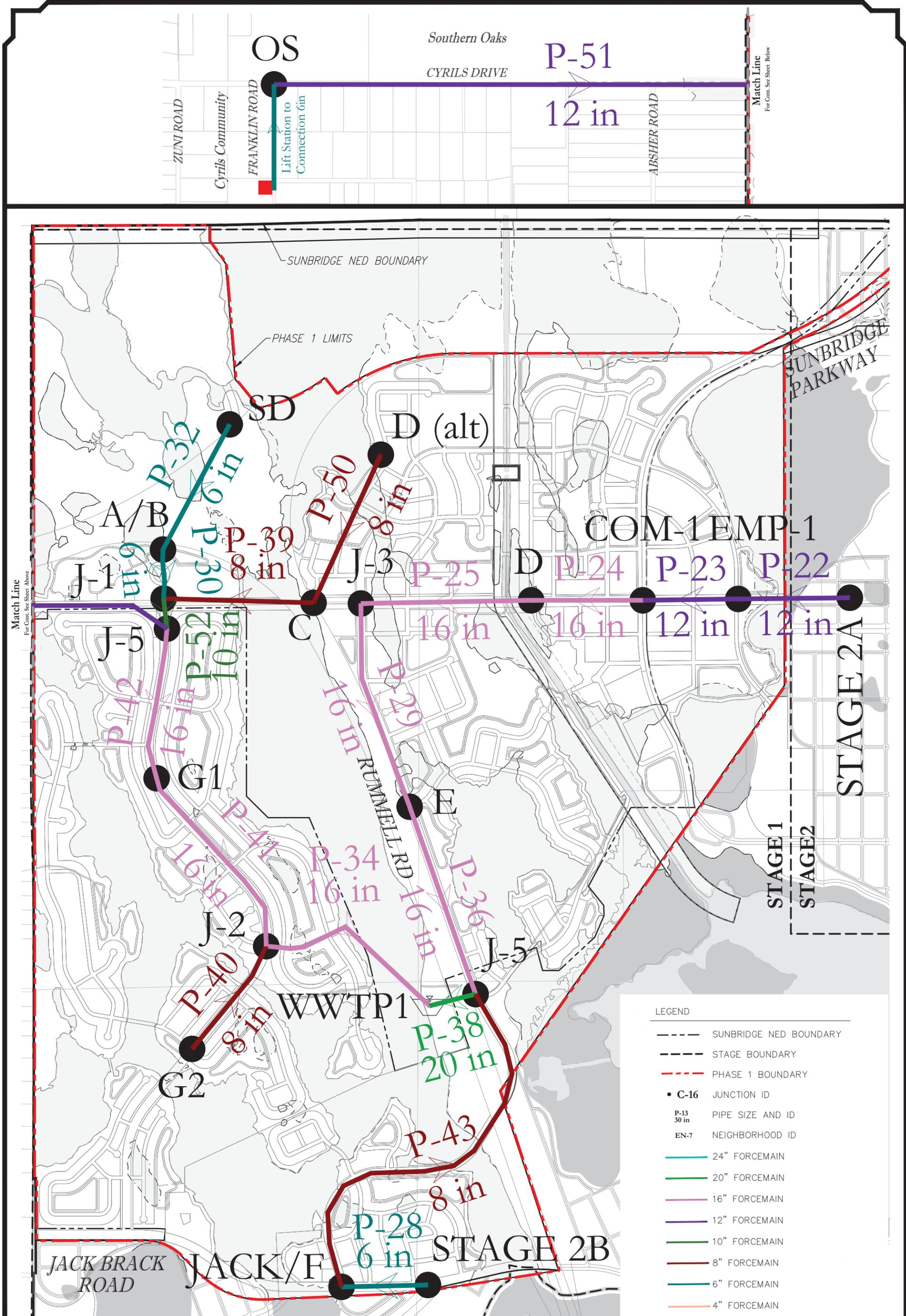
Figure 2-2. Sunbridge NED Phase I Wastewater Service Area
