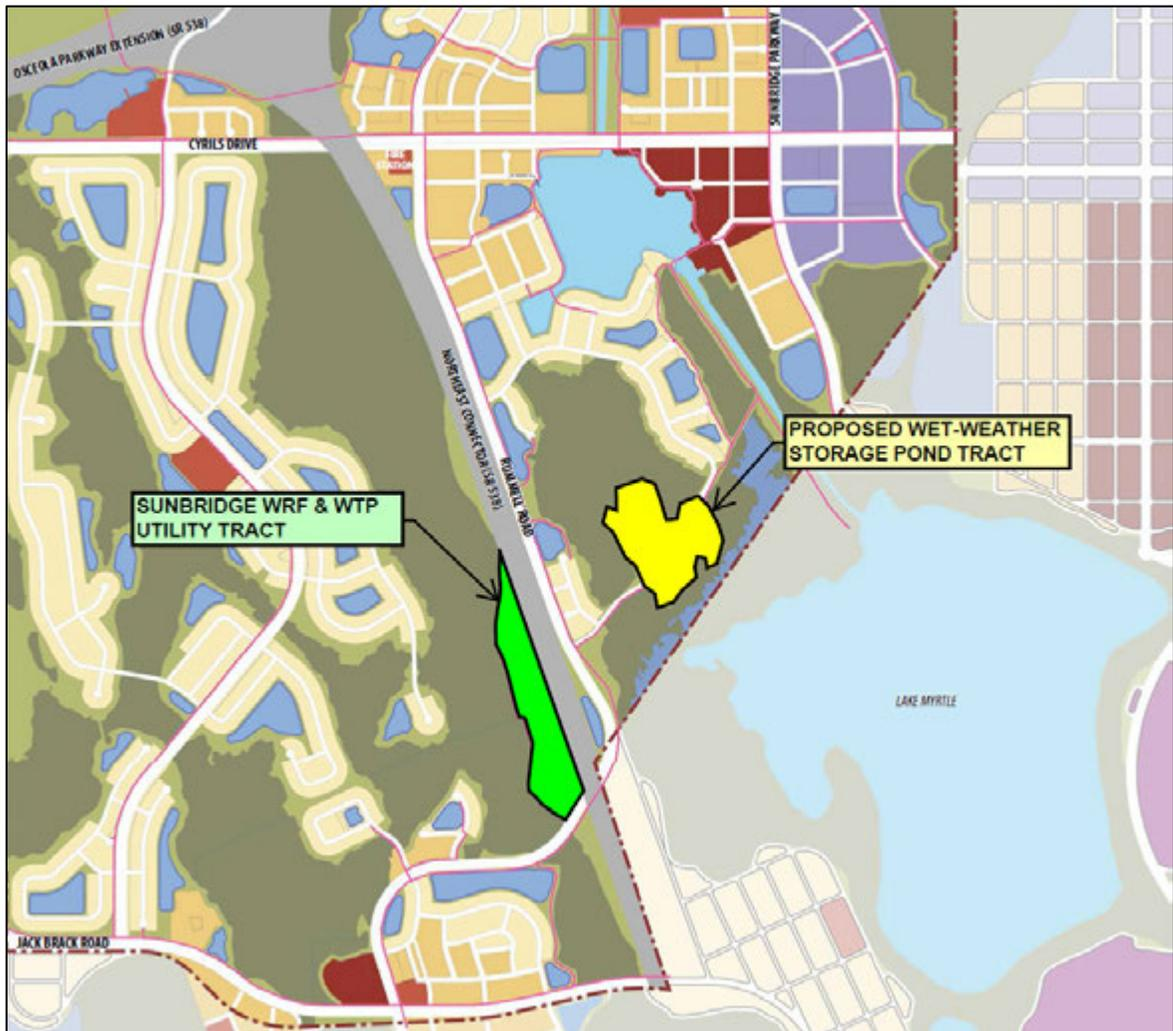
Figure 6-3. Proposed Wet-Weather Storage Pond Location
