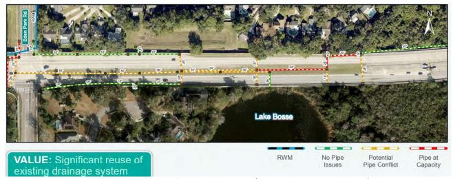
Figure 9. Transverse Stormwater pipes (Ex. near Eden Park Road)
