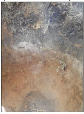
Figure 14. Typical soil profile in FPC Joel.
