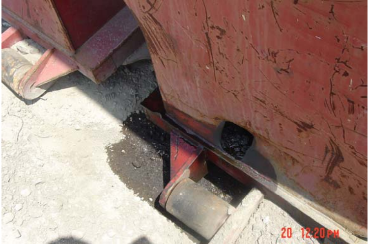
Fig. 7-Release from core parts in roll-off container.
