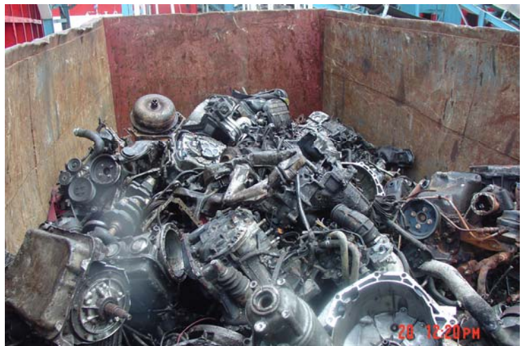
Fig. 6-Core parts stored in an uncovered roll-off container.
